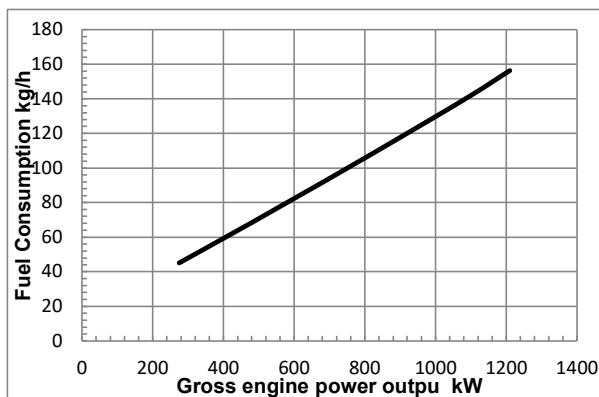
Curves shown above represent gross engine performance capabilities obtained and corrected in accordance with SAE J1995 conditions of 29.61 in. Hg(100kPa) barometric pressure [300ft.(91m) altitude] 77deg F (25 deg C) inlet temperature, and 0.30 in. Hg(1kPa) water vapor pressure with No. 2 diesel fuel or a fuel corresponding to ASTM D2.
